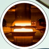
Produces ultrapure silicon crystal by the Float Zone (FZ) method
